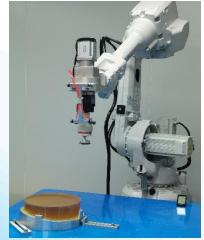
Computer Controlled Optical Surface (CCOS) polishing technology was adopted. According to the established mathematical model, the material removal amount is controlled by controlling the motion path, relative pressure and resident time of the grinding head on the machined surface. It has higher polishing efficiency than the traditional polishing process, and has higher surface shape accuracy index.
