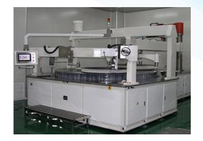
The most important feature of the ring polishing machine is high processing accuracy and outstanding efficiency, which can stably achieve the accuracy requirements of the large aperture component ( $\Phi$ 400-2000mm) surface shape 1/20 $\lambda$ . The products of the ring throwing machine have been put into major national projects in the fields of national defense and aerospace.
