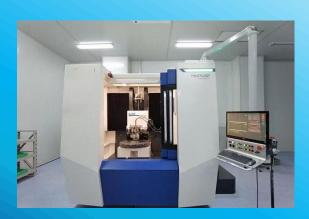
Magnetorheological Finishing (MRF) is an ultra-precision machining method using the rheological properties of magnetorheological polishing fluid in a magnetic field. The magnetorheological fluid is mainly composed of discrete micron magnetic particles, carrier fluid and surfactant. It has the characteristics of magnetic properties, rheology and stability.
